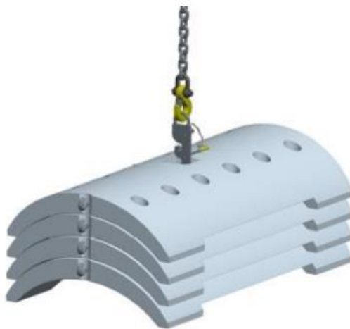
Plate 4-3: Typical Concrete Cover Installation
